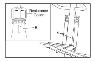
WARNING: The resistance cylinders become very hot during use. Touch only the resistance collars when changing the stepping resistance.
